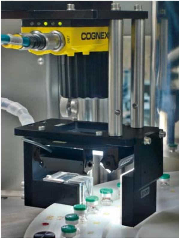
Cognex vision and ID technology helps companies improve their manufacturing quality and performance by eliminating defects, verifying assembly, and tracking and capturing information at every stage of production to ensure the entire process is completed correctly. And, Cognex read and verify solutions for mass serialization help achieve compliance with new product authentication and traceability requirements.
